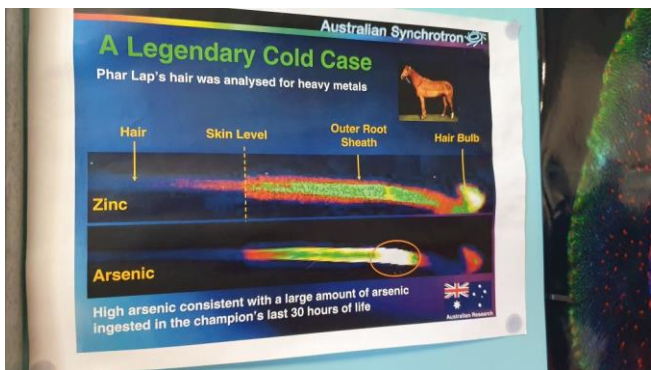
An example showing how the Synchrotron can be used analyse the chemicals in hair.
